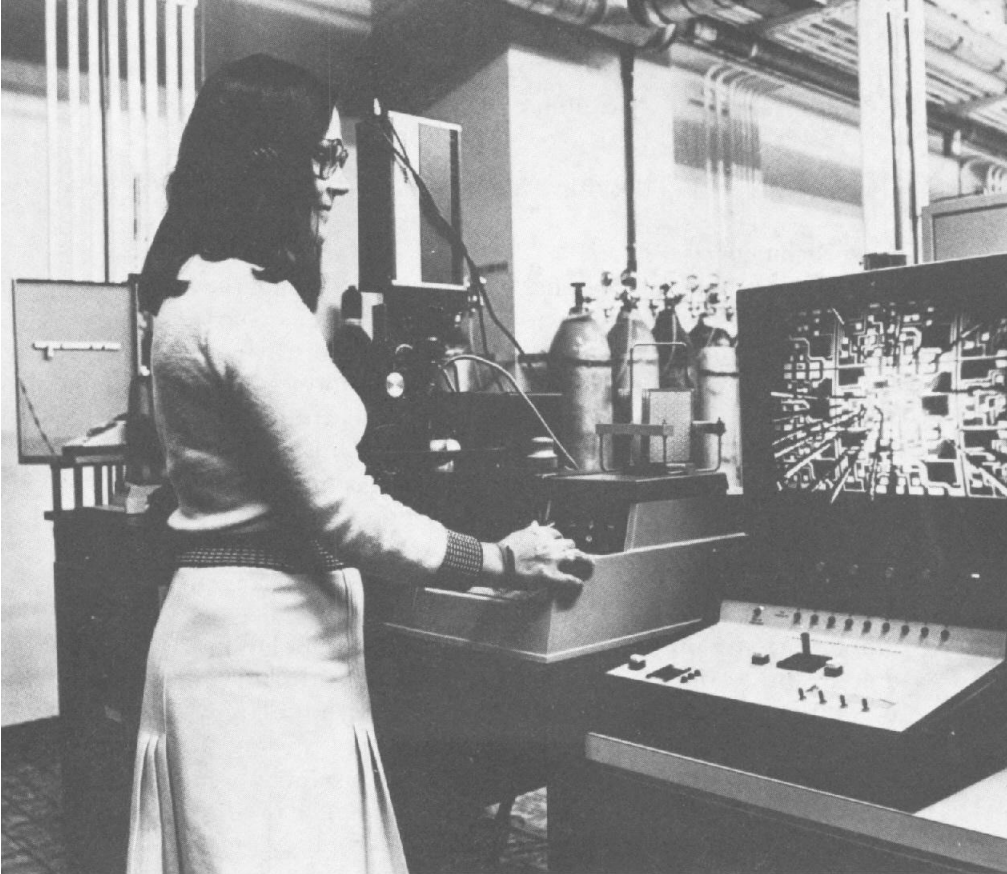
Adjusting integrated resistance by programmed laser beam, one of the new technologies being developed in Brabant Province Courtesy Belgium Information and Documentation Institute
